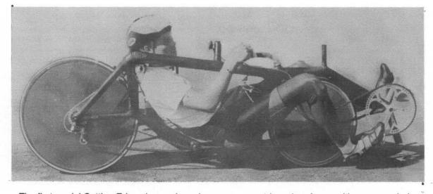
The first model Cutting Edge shown above has an asymmetric carbon frame with a suspended sling seat, stabilized by cross ties. The second model, as yet uncompleted, has a front-wheel drive.
