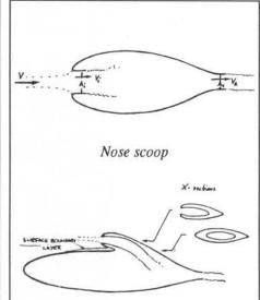
Side-scoop (The side scoop is <u>much</u> more difficult to design properly, and may trigger external separation on the aft body. The nose scoop is almost foolproof by comparison.)
