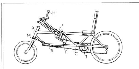
Figure 1 Elevation drawing of the leg-assist rowing bicycle
