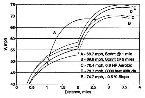
Several variations of the sprint are illustrated such as: (A) starting the sprint at one mile, (B) starting at 2 miles, (C) increasing aerobic output to 0.6 hp prior to sprinting, (D) increasing altitude from sea level to 8000 feet, and (E) running on a constant 0.5% downhill. It is interesting that the 0.5% downhill does more for increasing velocity than the 8000 foot altitude (air density = 0.001869
