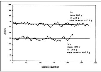
Figure 4. An example of the data stream from the force balance
