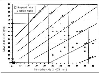
Figure 2. Dish ratio □ drive side/non-drive side
