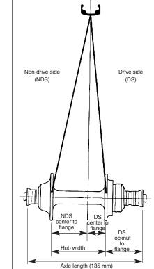
Figure 1. Wheel dish. This diagram appears in The Bicvcle Wheel and is used with the author's permission.
