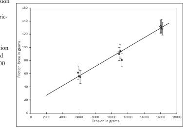
Figure 2. Friction on the 42-tooth sprocket
