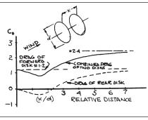
Figure 1. Interaction between two disks placed one behind the other
