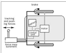
Figure 3. Function structure of the phantom trailer
