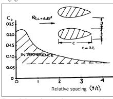
Figure 6. Drag of a pair of struts, one beside the other.
