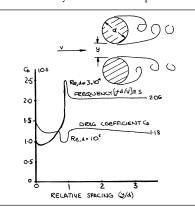
Figure 5. Drag (and vortex-street frequency) reference of a pair of circular cylinders placed side-by-side.
